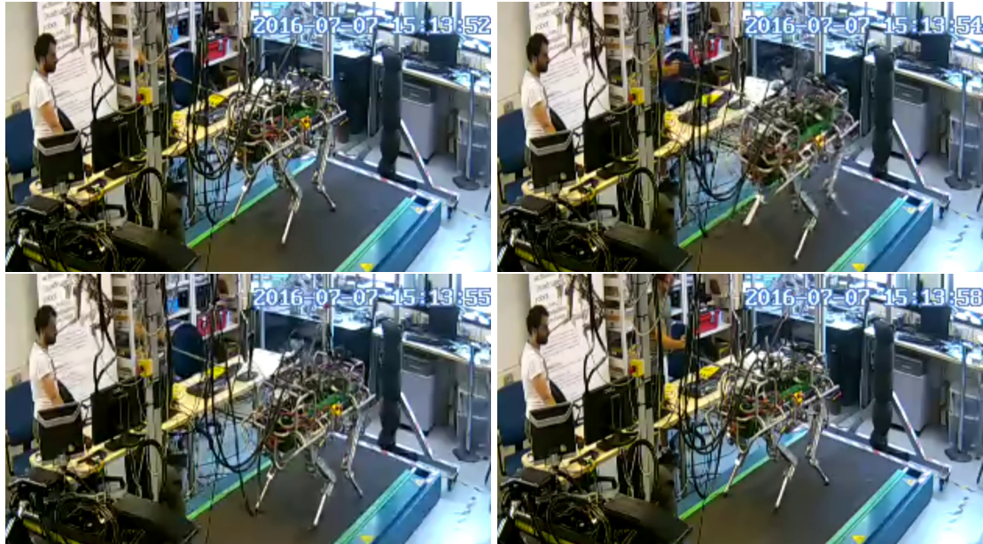
Figure 5.8: Push recovery with state estimation in the loop. The robot was commanded to trot in place and keep its position. After several pushes from the operator, the robot recovered its position along the green line of the treadmill. The ability to recover its position in a constrained space using the state estimation in the loop demonstrates the reliability and robustness of the filter.
