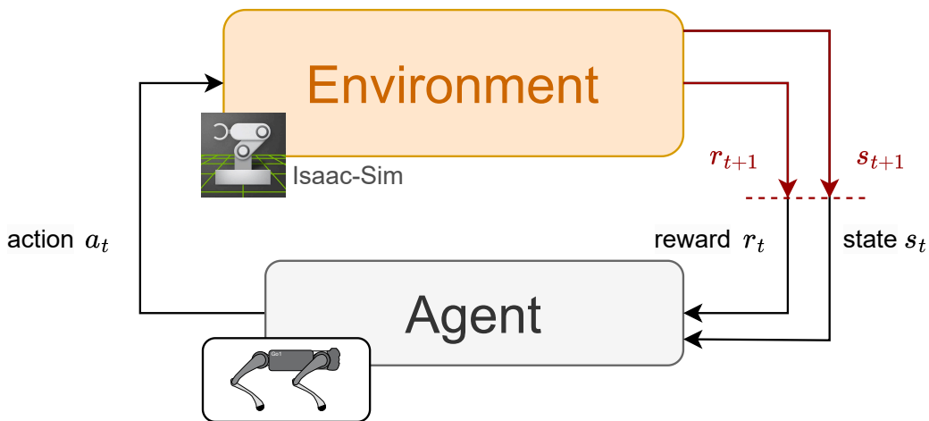
Figure 2.2: Interaction schema between the Go1 robot (agent) and Isaac Sim (environment), showing the exchange of actions, state, and rewards between these two entities
