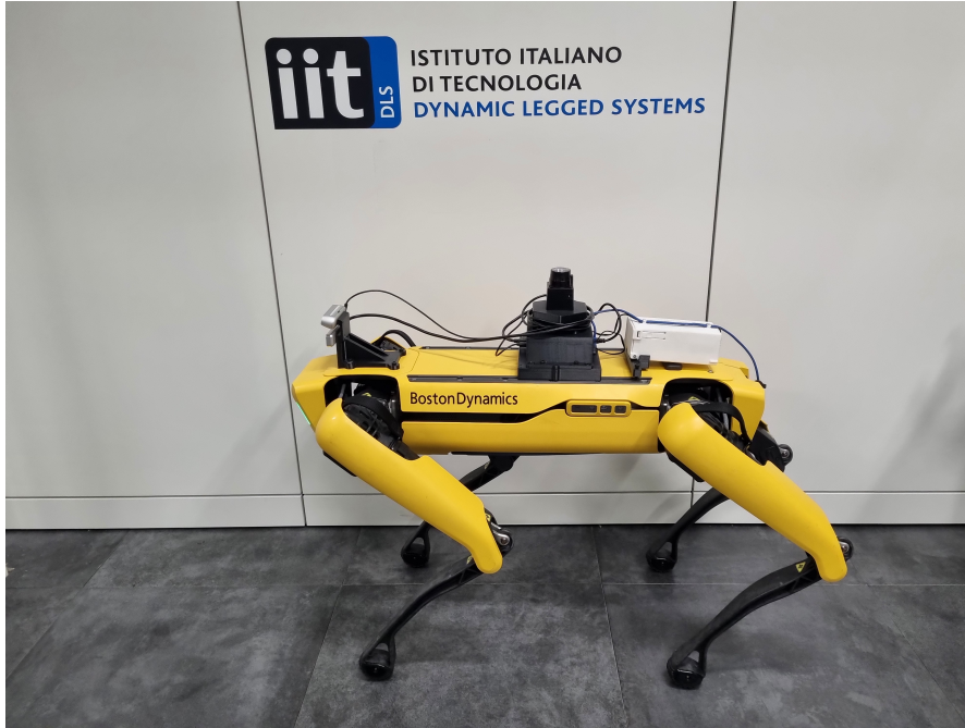
Figure 1.2: Our quadruped platform: Boston Dynamics Spot with the onboard computer and sensor payload used in this thesis.
