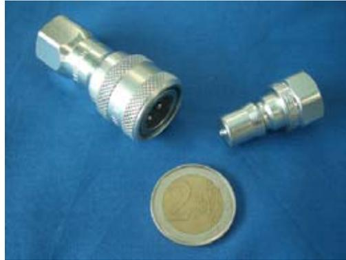
**Figure 4.19:** Pictures of *Faster* quick release coupling, size 1/8inch, with a 2Euro coin (diameter 26mm) as reference.
