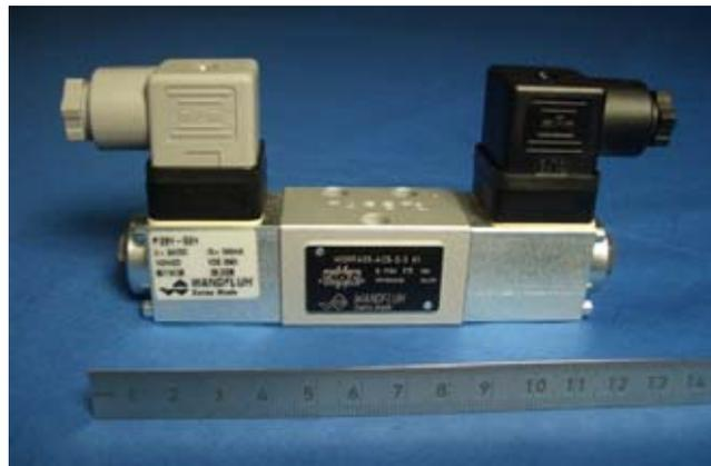
**Figure 4.15:** Picture of the proportional spool valve *Wandfluh WDPFA03-ACB-S5-G24* with a metric ruler with centimetres.
