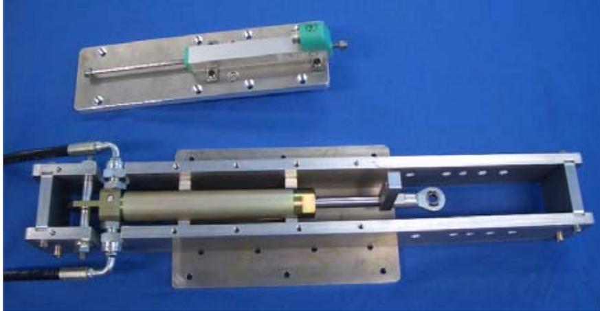
**Figure 5.3:** Picture of the hydraulic cylinder test bench, showing the base with cylinder in the bottom of the picture and the top part with linear potentiometer in the top of the picture.
