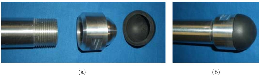
**Figure 4.8:** Pictures of the basic HyQ foot: **(a)** disassembled and **(b)** assembled.
