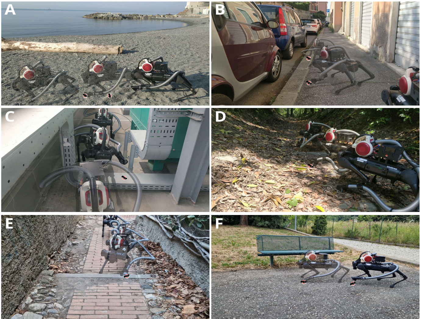
Fig. 7. The prototype has been tested successfully in six different scenarios. Starting from the top left corner, we show the robot, controlled with a joystick for safety reason, traversing environments named beach (A), urban (B), industrial (C), natural (D), non-flat (E) and park (F). All these scenarios are characterized by unique challenges both from the locomotion point of view, such as stairs and slopes (scenarios A, D, E, and F), and from the detection point of view due to the presence of similar objects in size and color (e.g. small leaves in scenarios D and F).
