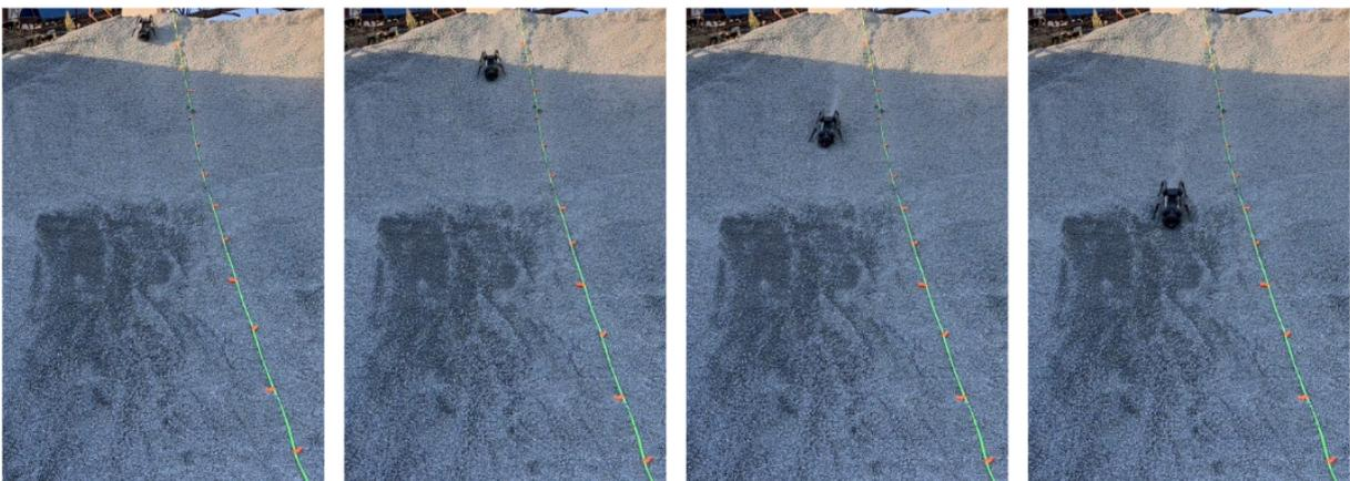
Figure 7. Image sequence of experimental trial of the Aliengo quadruped robot with custom-designed lower torso (version 3) sliding down an approximately 10m tall pile of pebbles without the need of swimming motion (from left to right, time between frames: 1.25s).
