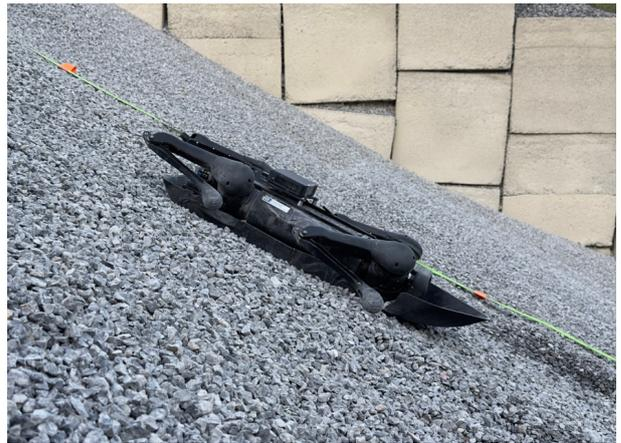
Figure 1. Picture of the Aliengo quadruped robot with novel, custom-designed torso (design 2) lying on a pile of pebbles with retracted legs.
