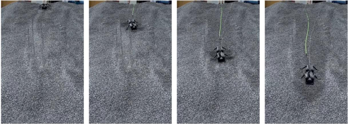
Figure 5. Image sequence of experimental trial of the Aliengo quadruped robot with custom-designed lower torso (version 1) sliding down an approximately 10m tall pile of pebbles with the help of swimming motion (from left to right, time between frames: 4s).
