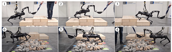
Fig. 8: Sequence of numbered snapshots from the HR collaborative carrying experiment transporting a rigid 7kg payload.
