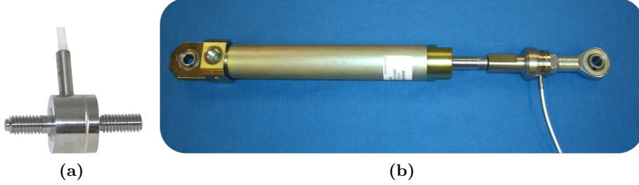
Figure 3.10: The HyQ load cell, shown in (a), is able to measure axial forces in the range of -5000\text{ N} to 5000\text{ N} . In (b), the HyQ cylinder is connected with the load cell in series with the rod.
