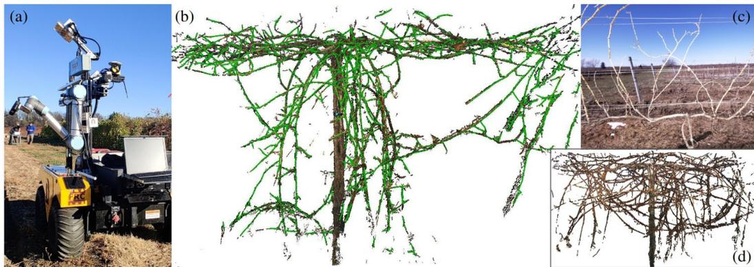
Figure 2.13 (a): Data collection robot. (b) Point cloud with overlaid skeleton data. (c) Simple grapevine used for robotics research. (d) A complex example of vines in real situations. (Obtained from Schneider et al., 2023)
