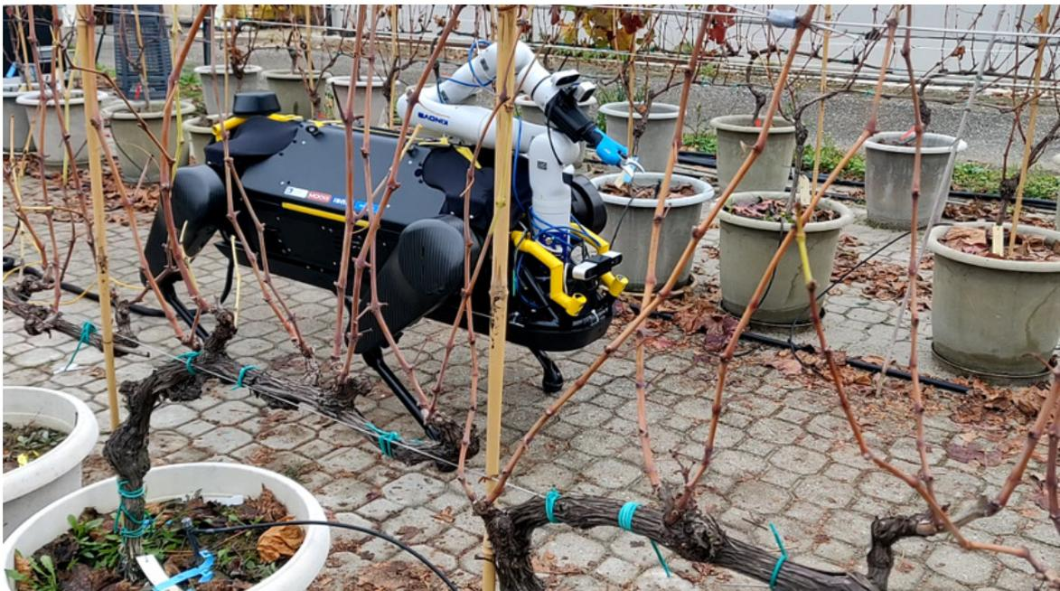
Figure 2.20 IIT's quadruped robot *HyQReal* (Semini et al., 2019) with Kinova Gen3 with seven DoF arm and pruning end effector.
