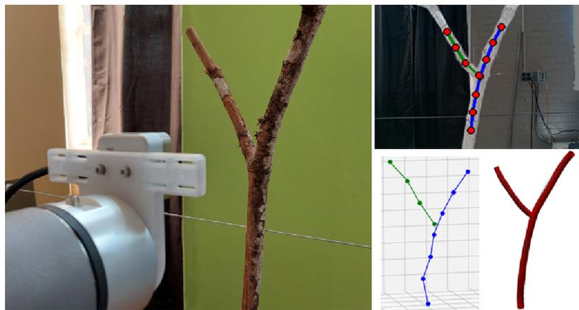
Figure 2.14 On the left, the robot along with the branch to be reconstructed, and on the top right, the extracted 2D points of interest, and bottom right presents the triangulation along with the branch 3D reconstruction. (Obtained from You et al., 2023)
