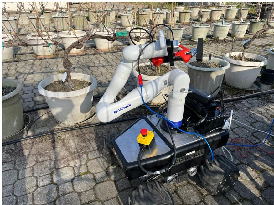
Figure 2.21 *Summit XL* with *Kinova Gen3 with seven DoF* and pruning end effector.
