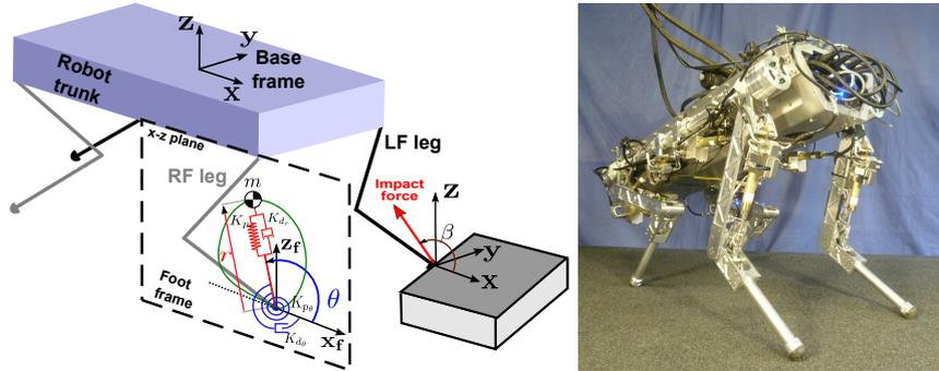
Fig. 1. **(Left)** The reflex trajectory, if restricted to the  $X - Z$  plane, can be described with radial  $r$  and angular  $\theta$  coordinates. The angle  $\beta$  of the impact force (see left-front leg) is expressed in the  $X - Z$  plane. **(Right)** Picture of the HyQ robot.
