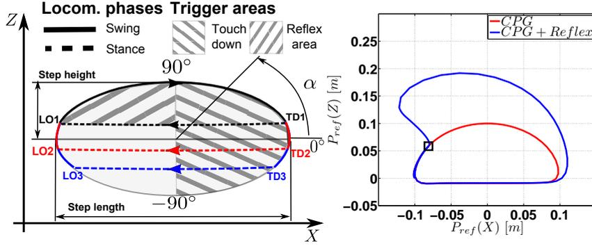
Fig. 2. **(Left)** Areas of the CPG cycle where a possible impact can trigger the limb reflex or the touchdown.  $\alpha$  is the phase angle of the CPG trajectory.  $TD_i$  are different touch-down events that result in different stance trajectories.  $LO_i$  are the correspondent lift-off events. **(Right)** Periodic foot (clockwise) trajectory (red), and the same trajectory modified by the reflex action (blue) for overcoming a frontal obstacle. The black square indicates the collision point.
