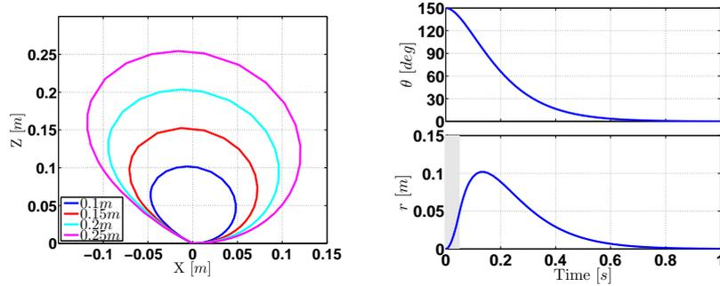
Fig. 3. Simulation. **(Left)** Reflex trajectory (clockwise) in the  $X - Z$  plane for different maximum retraction values. **(Right)** Time response of the polar coordinates ( $t_{rfx} = 0.5s$ ,  $r_{max} = 0.1m$  and  $\theta_0 = 150^\circ$ ). The shaded area highlights the interval during which the retraction impulse is acting.
