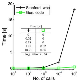
Fig. 6. Performance comparison with the *S-wbc* for the computation of the inverse of the joint space inertia matrix  $M^{-1}$  and the end-effector Jacobian  $J$ , for a 5 DoF robot. The  $x$  axis represent the number of calls to the update functions  $M(\mathbf{q})^{-1}$  and  $J(\mathbf{q})$ , the  $y$  axis the total execution time in seconds. The same random joint state vector  $\mathbf{q}$  is used for each call on both implementations.
