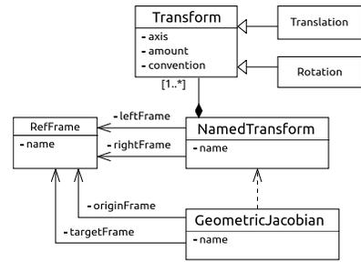
Fig. 3. The model of coordinate transformations and Jacobians as an UML class diagram. Transforms are composition of basic rotations and translations; named transforms describe the relative pose of two known frames; left and right refer to the position of frames B and A in the notation  ${}_B X_A$ . Jacobians on the other hand are fully determined by a pair of frames, as they can be computed from the transformations related to such frames.
