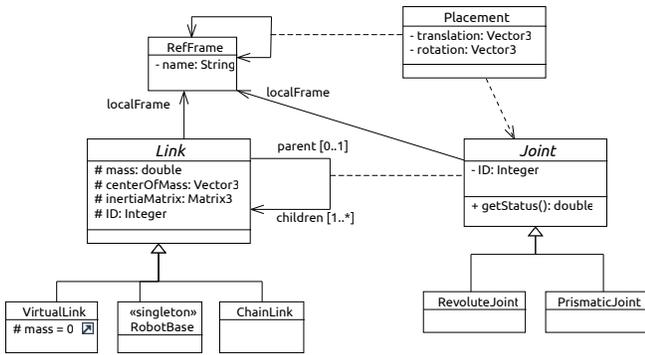
Fig. 1. The kinematic tree (meta)model as an UML class diagram. It can represent a tree-like layout of rigid bodies, capturing the role of joints as the connection between any pair of parent/child bodies, and emphasizing their association with reference frames. The convention about the placement of these frames and numerical data about the relative pose of two successive ones (the Placement class) provide the full geometry information about the robot.
