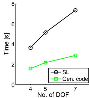
Fig. 5. Performance comparison with the SL software about the Newton-Euler algorithm for inverse dynamics. The plot shows the cumulative execution time for  $10^6$  calls of the function  $\tau = f(\dot{q}, q, \dot{q})$  as a function of the number of degrees of freedom of three robot models.
