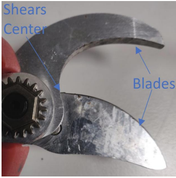
Fig. 2. Picture of commercial pruning blades with the definition of the Shears center.
