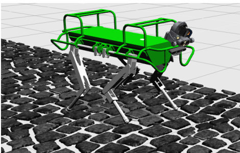
Fig. 1: The HyQ robot trotting on cobblestones in simulation.
