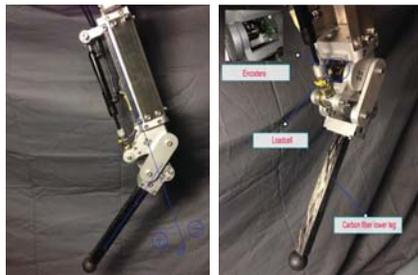
Fig. 10. Hardware implementation. *Left*: Side view of the *isogram mechanism* based knee joint; *Right*: close up view of load cell and encoders.
