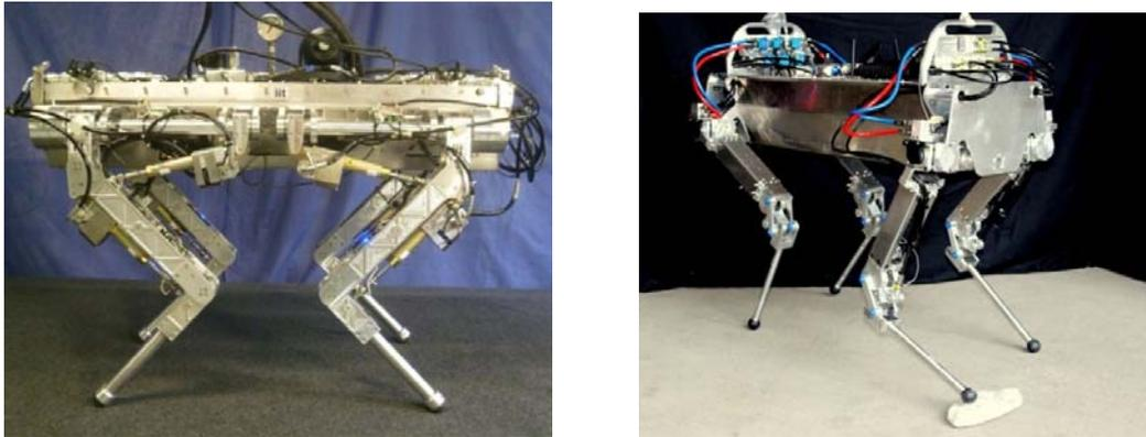
Figure 1. The DLS lab robots (*left*) the HyQ Robot; (*right*) the MiniHyQ Robot
