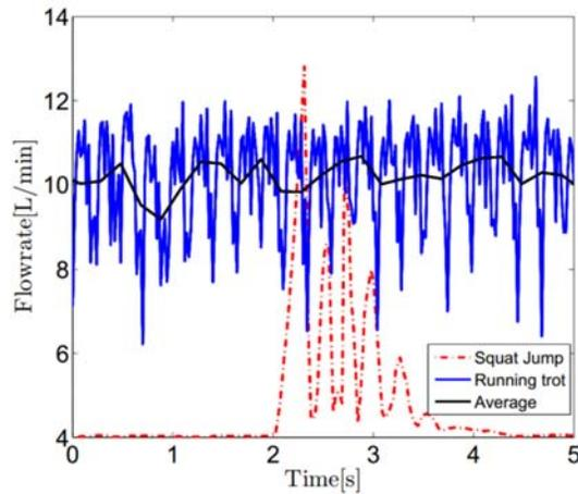
Figure 6. Estimated flow rate, blue line shows the total required flow rate of the robot while Running trot, red dotted line shows the total required flow rate while Squat Jump, and black line shows the average flow rate while Running trot.
