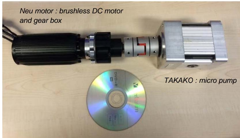
Figure 8. Picture of chosen pump and electric motor with a standard-size compact disc to indicate the size
