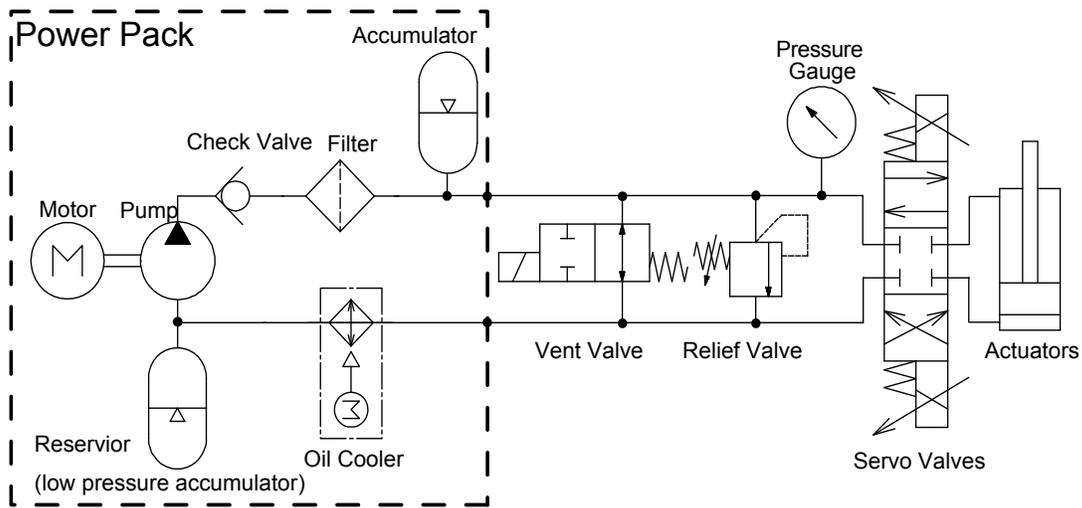
Figure 5. Schematic of Hydraulic system
