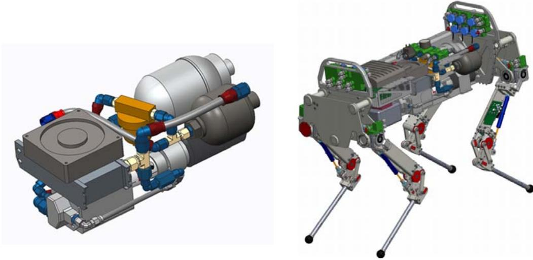
Figure 4. The CAD model of MiniHyQ with exposed view of onboard power pack, magnetic encoder disks and EtherCat control PCB in upper leg link.
