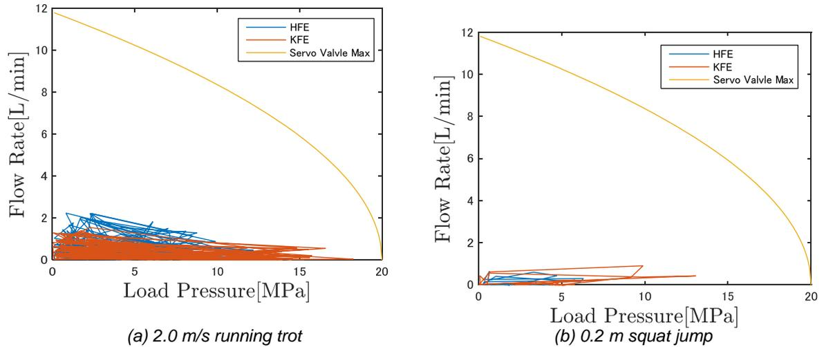
Figure 7. Verification of servo valve performance
