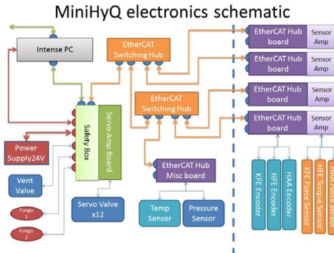
Figure 3: MiniHyQ's control system architecture
