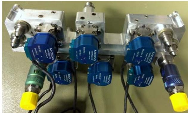
Figure 9: MiniHyQ's centralized manifold
