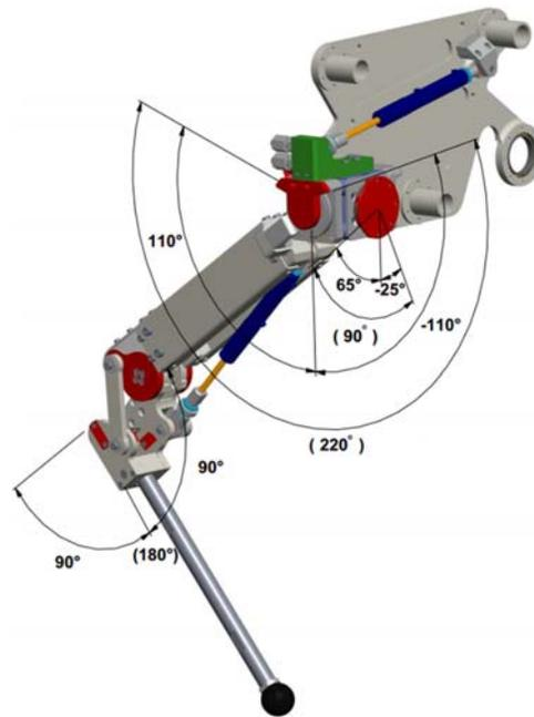
Figure 2. CAD model of MiniHyQ Leg which is consist of 3 active DoF i.e HAA, HFE and KFE joints.
