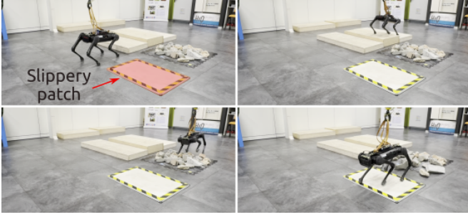
Fig. 3: During the closed-loop experiment, Aliengo walked up and down the stairs, then on rocks and slippery terrain, repeating these tasks three times.
