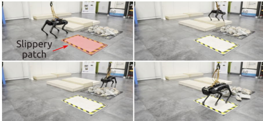
Figure 4.8: Aliengo in a closed-loop experiment: During the closed-loop experiment, Aliengo walked up and down the stairs, then on rocks and slippery terrain, repeating these tasks three times.
