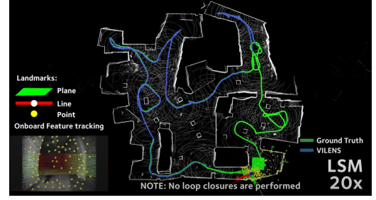
(b) Vilens was tested on several Dataset. This image shows the results obtained from the LSM Dataset of the Urban Circuit of the DARPA SubT Challenge [89].
