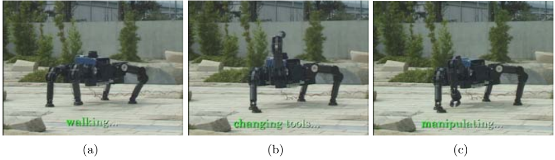
Figure 2.18: TITAN-IX demonstrating (a) walking, (b) changing tool and (c) manipulation task capabilities
