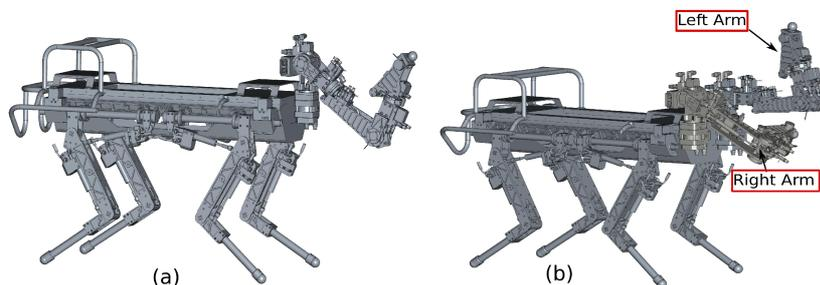
Figure 6. Future work: (a) The HyQ robot with the HyArm (b) The HyQ with dual arm system (Centaur robot)
