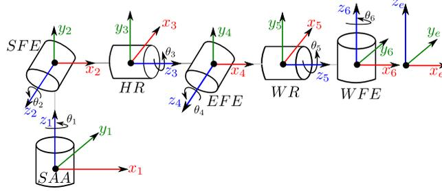
Figure 3. HyArm kinematics: Shoulder Adduction/Abduction (*SAA*), Shoulder Flexion/Extension (*SFE*), Humerus Rotation (*HR*), Elbow Flexion/Extension (*EFE*), Wrist Rotation (*WR*), Wrist Flexion/Extension (*WFE*) All the joints are shown at zero configuration
