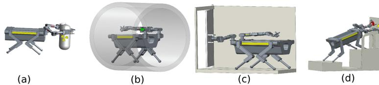
Figure 1. Conceptual tasks for the centaur robot (a) Carrying an object (b) Passing through a narrow passage (c) Opening a door (d) Body stabilization of the robot
