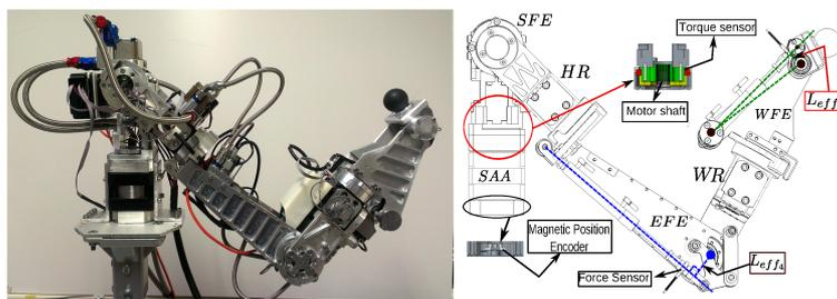
Figure 2. The HyArm: (left) Real robot side view (right) CAD model showing actuator arrangement (see section 4 for further details)
