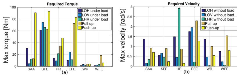
Figure 5. (a) Required torque and (b) velocity for lifting an object, biceps curl, pull-up and wall push-up tasks for each arm joint. LO:Lifting an Object, V:Vertical, H:Horizontal, HR:Humerus Rotation
