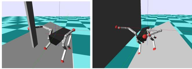
Figure 4. Picture of the Centaur simulation during the pull-up (left) and push-up (right) tasks.
