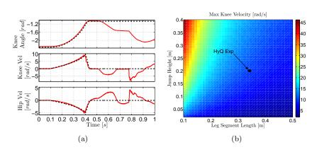
Fig. 3. (a) Plot of experimental data (red solid) and simulated data (black dashed) for a squat jump motion of 0.2m jump height. *Top:* knee joint angle  $\theta_2$ ; *middle:* knee joint velocity  $\dot{\theta}_2$ ; *bottom:* hip joint velocity  $\dot{\theta}_1$ . (b) plot of maximum knee joint velocity for different leg segment lengths and jump heights. The arrow marked with *HyQ Exp* shows the experimental results obtained with HyQ as an example.
