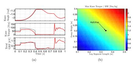
Fig. 2. (a) Plot of experimental data (red solid) and simulated data (black dashed) for a squat jump motion of 0.2m jump height. *Top:* knee joint angle  $\theta_2$ ; *middle:* knee torque  $\tau_2$ ; *bottom:* total ground reaction force  $4F_{zf}$ . (b) plot of maximum knee joint torque scaled by the robot's body weight (BW) for different leg segment lengths and jump heights. The arrow marked with HyQ Exp shows the experimental results obtained with HyQ as an example.
