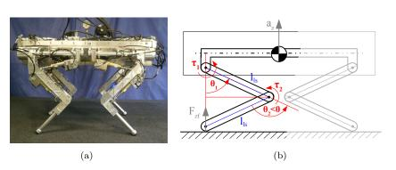
Fig. 1. HyQ: Hydraulic Quadruped robot. (a) picture and (b) sketch of side view of robot in squat posture, defining the centre of mass (COM) acceleration vector  $a_z$ ; joint angles  $\theta_{1,2}$  and torques  $\tau_{1,2}$  of the hip and knee joint, respectively; leg segment lengths  $l_{ls}$  and ground reaction force vector at the foot  $F_{zf}$ .
