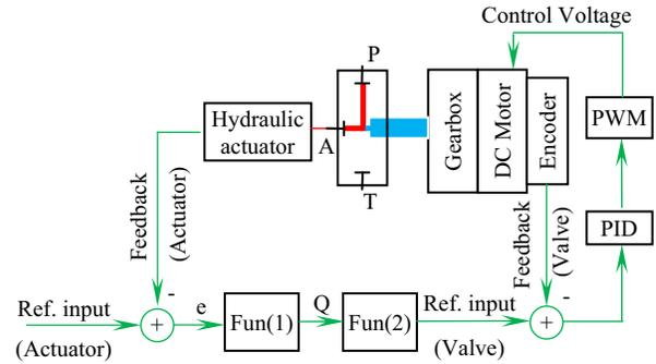
Fig.2 Operating principle
