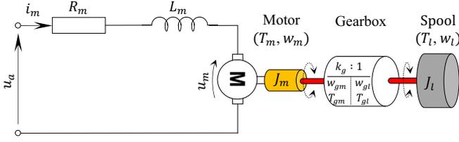
Fig.4 Model of the rotary valve
