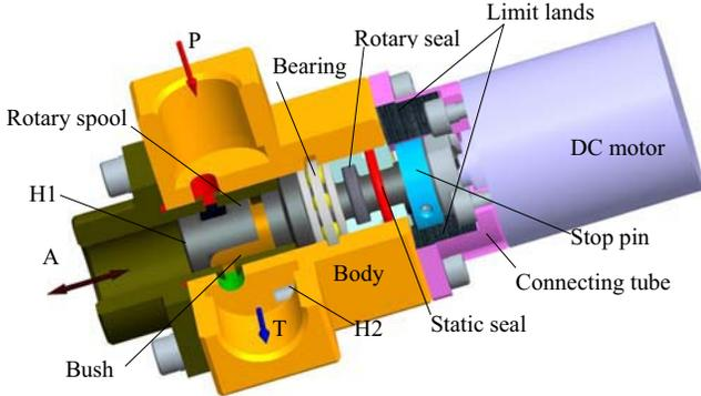
Fig.1 Schematic of DC driven rotary spool valve
