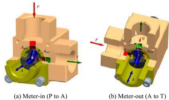
Fig.9 Flow induced torque
