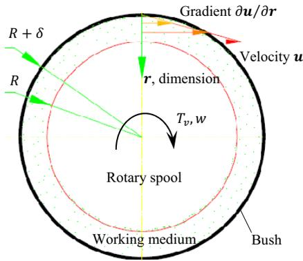
Fig.6 Laminar shear of the fluid between the spool and bush
